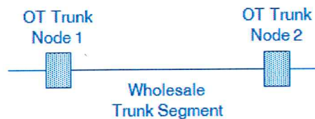
Figure 3-1 Trunk Segment of Leased Line
